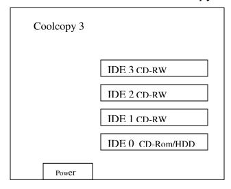
When the system connects with the hard drive, the hard drive must connect on the IDE 0 port with the "Master" setting and the CD-ROM must set at "Slave".
